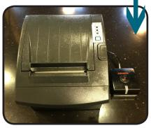
The OLO printer is a standard Espon printer that included a button that makes a sound when an order is recieved.
